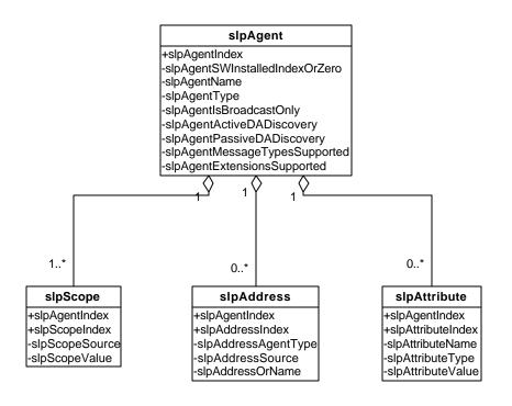
This UML object model is for use in discussing the content of an SLP MIB. It is an abstract model; each of the objects shown here is represented in the MIB by a set of tables. For clarity, not all attributes are shown, and no statistics are specified. In the event that these objects do not match the MIB, the MIB is the final authority.
